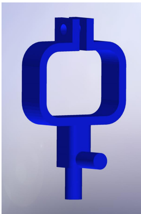
Figure 1 Technical project for 3D printing of the device that connects the hydraulic arm to the ultrasound transducer.
